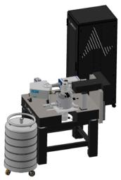
The **Allalin 4027** is a nanometer resolution spectroscopy instrument, based on a disruptive technology called low-temperature quantitative cathodoluminescence, that tightly integrates a scanning electron microscope, a light microscope and a cryogenic stage into one tool. It is designed for those who need to follow a tight technology roadmap and quickly access to extremely precise spectroscopic information that has been unavailable from traditional techniques.
