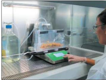
New standards make it necessary to work under a laminar flow for the dilution work, and this can create operational problems.
