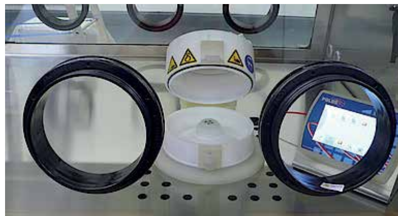
Picture shows Jacomex glove box with a SPIN150i integrated
