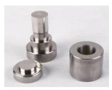
Fill the fine powder samples after grinding into the specified stainless steel ring. Moving the ring with samples to the beneath of press plunger and pressing is started. During pressure build-up the density of the powder increases. The max. pressure maintained for a period of time to increase interparticle adhesive force to ensure the max. stability of the tablet.
