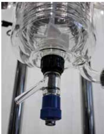
Pressure Sensitive Spring Loaded Flush Valve Prevents Leakage
