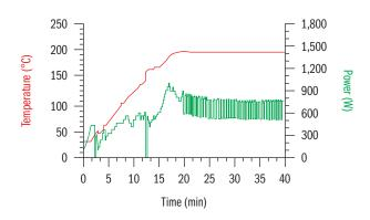
iWave sensors allow for fine power control, as shown in this graph. Temperatures can then be held tighter and digestions are more reproducible.
