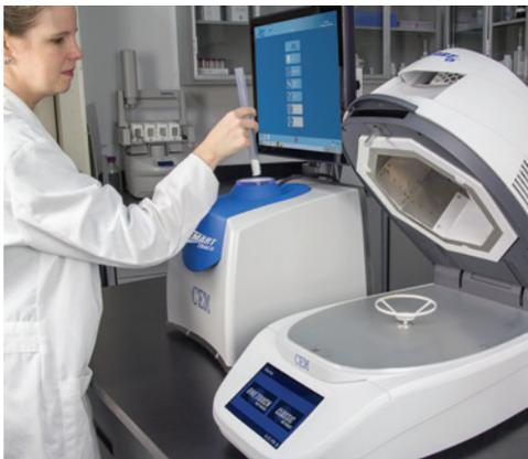
The SMART Trac II partners advanced, high performance NMR technology with the fast, reliable drying capability of the SMART 6 Moisture/Solids Analyzer to create a system which yields fast, accurate results without solvents or calibration. The **speed** of iDri™, the **versatility** brought by iPower®, and the **accuracy** that is available when using AOAC approved methods make the SMART 6 the best way to directly determine and remove moisture prior to fat testing.
