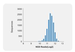
12,000 unique oligos synthesized on semiconductor chip result in ~100% oligo coverage with interdecile ratio of 1.98
