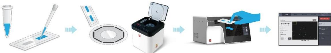
Counting with the QUANTOM Tx Microbial Cell Counter
