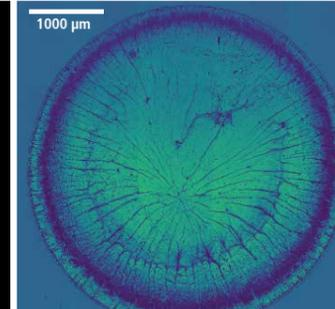
Drying of a sessile droplet of a graphene dispersion
