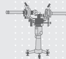
A mapping ellipsometer is a non-imaging ellipsometer with a motorized stage. Psi and delta readings are measured at one spot and then the table is moved to another sample location and the process is repeated until enough data is collected to construct a
