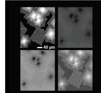
Ellipsometric contrast micrographs of CWD graphene
