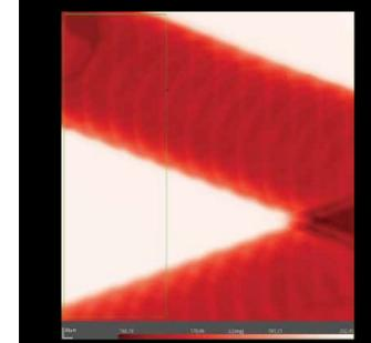
Film thickness of ALD-printed thin film structures
