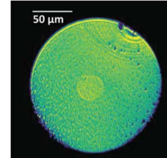
Air | As<sub>2</sub>S<sub>3</sub> (fiber, core/clad)
