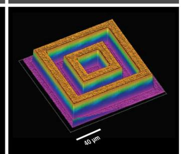
Microscopic maps of oxide layer thickness
