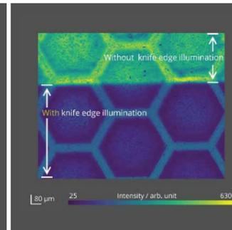
Honeycomb-like coating on glass: improved imaging with knife edge illumination
