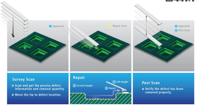
Following the repair, Park NX-Mask employsour non-contact AFM technology to conduct post-repair verification, generating nanoscale 3D topography and other critical metrology data such as surface roughness.
