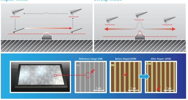
Photomask defects are a result from foreign particles in the environment or by erroneous pattern processing. The most commonly found defects on high-end photomasks are tin particles generated during the EUV lithography process. The AFM nanomechanical method of Park NX-Mask offers many advantages that are superior and completely safe for photomask repairs.
