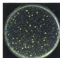
A measurement of general viable bacteria. All colonies in the measurement area were counted.
