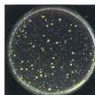
A measurement of general viable bacteria. All colonies in the measurement area were counted.
