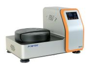
The grinding jar is arranged on the sun wheel of the planetary ball mill off centered. The rotate direction of the sun wheel is opposite to that of the grinding jar in a ratio of 1:-2. The velocity difference between the ball and the grinding jar creates an interaction force of friction and impact, which releases high dynamic energies that act on the particle sample so as to quickly produce highly uniformed and very fine particle.
